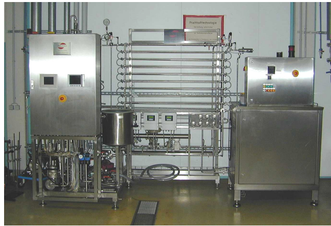
Tubular heat-exchanger used for controlled continuous thermal treatments of purées and juices at pilot-plant scale.
